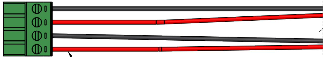
1401.E.013.V1.00 - BATTERY HARNESS 4 WIRES - RED AND BLACK SAP NUMBER: WH1401E01300
